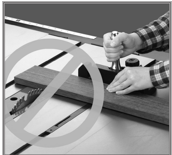
Figure 3. Do not make through cuts without the blade guard/splitter or riving knife in place.
